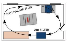
currents can be seen on a bright sunny day, when there are a lot of fine dust particles in the air. Mounting the unit this way will increase efficiency.
